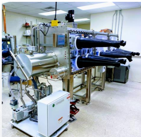
2 triple workstation inert atmosphere gloveboxes
