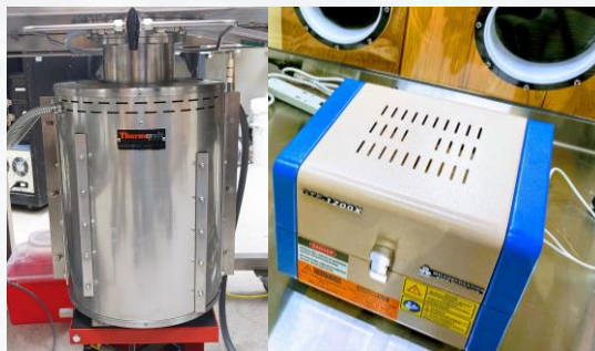
Furnaces & induction heater max. temp. 1000-2000 °C
