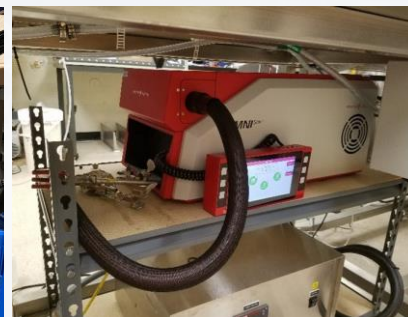
Gas analyzer ( \geq 100 ppb) plumbed to glovebox
