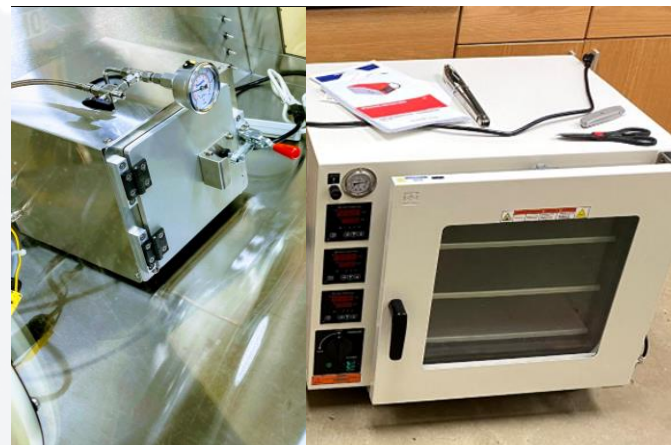
Vacuum drying ovens in and out of glovebox (up to 300 °C)
