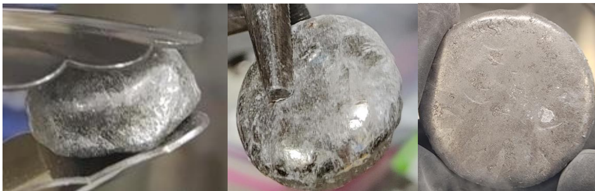
Figure 2: Ingot recovered from run Ce-1 using an \text{Al}_2\text{O}_3 crucible (left). Ingot recovered from run Ce-2 using an yttria-coated \text{Al}_2\text{O}_3 crucible (middle). Ingot recovered from run Ce-3 using a \text{MgO} crucible performed at a larger scale (right).
