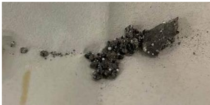
Figure 10: Photo of cathode deposit from run In-1.
