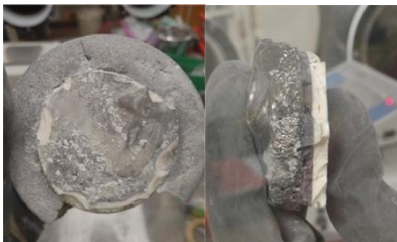
Figure 5: Bottom view of electrorefining crucible with the base of the outer crucible removed showing that no cathode ring was obtained from run Ce-4 (left); anode leftover from run Ce-4 (right).
