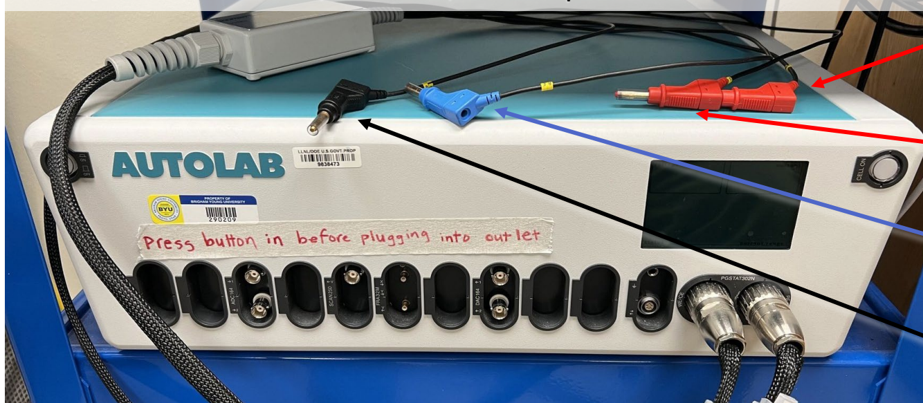
Potentiostat with RE/CE and S/WE coupled for 3-Electrode Cell
