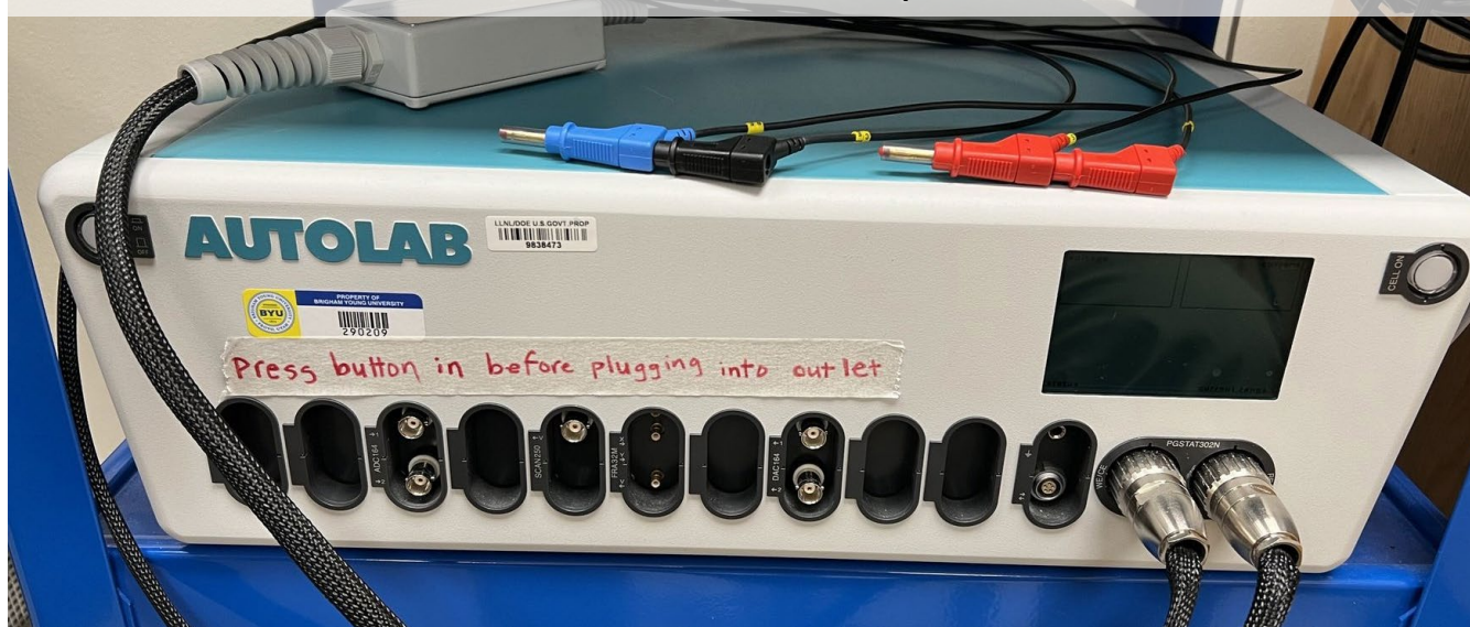
Potentiostat with RE/CE and S/WE coupled for 2-Electrode Cell
