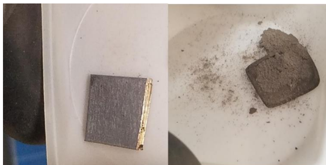
Figure 12. Ce foil before (left) and (after) chlorination.
