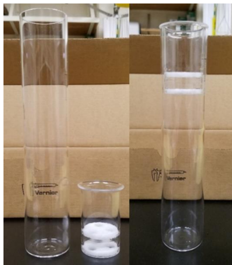
Figure 5. Quartz Crucible and Basket. Side-by-side (left) and nested (right) views.
