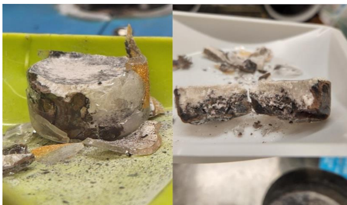
Figure 13. Salt block after REE chlorination experiment. Full block (left) and bisected (right).
