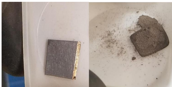
Figure 12. Ce foil before (left) and (after) chlorination.
